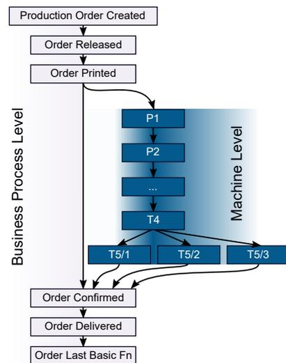
Fig. 1. Target process model of the considered multi-level interlinked manufacturing process.
