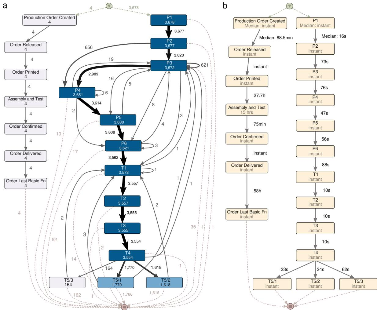
Fig. 3. (a) Process map of the multi-level interlinked manufacturing process as it is actually executed. The map was created with the PM tool Disco. The arcs are labeled with the number of orders or respectively valves passing the process steps. (b) Filtered target process. The process map includes statistics of the process execution. (An artificial bias was added to all statistics for confidentiality reasons.)
